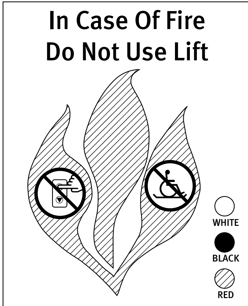
Figure 2.6.7.2 Platform Lift Corridor Call Station Pictograph
